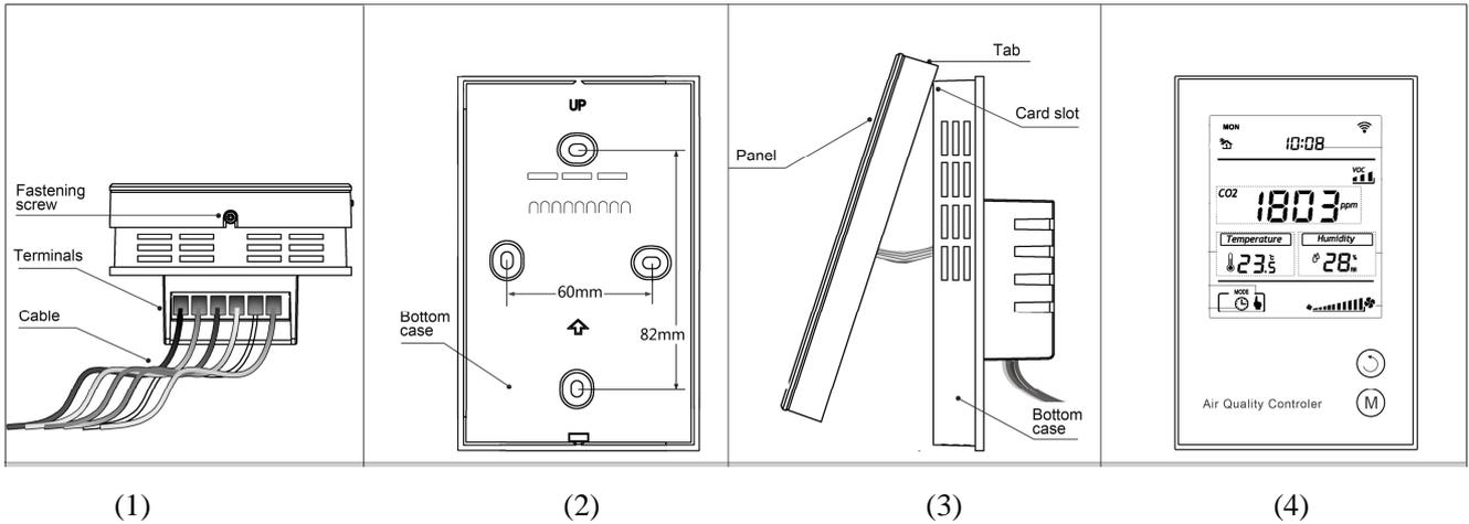
**Step 1:** Separate Panel and Bottom case by removing the screw at the bottom of device. Insert all wires into the right terminals and tighten screws. The wiring diagram is shown above.
